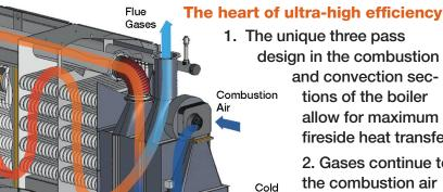
1. The unique three pass design in the combustion
